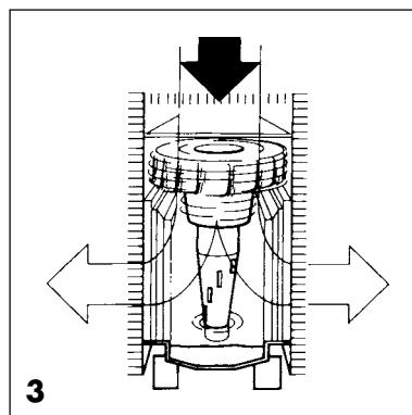
When the actual value (e.g. 40) is less than the reference value (e.g. 45), the appliance humidifies the room air and purifies it simultaneously.
