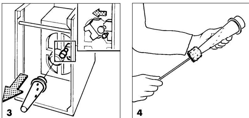
**Fig. 5** PH14: Clean the evaporator mat, droplet trap, mobile base cover and mobile base.
