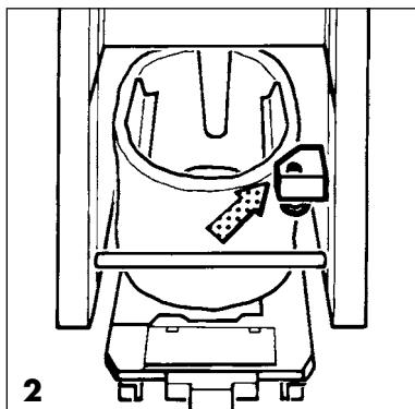
**Fig. 3** Locate the cross bar exactly in the recess.
