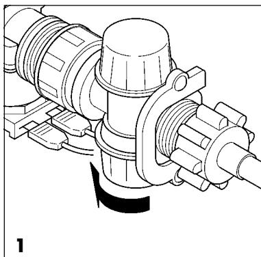
**Fig. 2** When replacing the appliance housing, take care that the level switch cover on the Quattro filter slides past freely.
