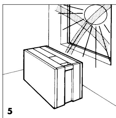
Move the PH14 carefully. Do not lift the appliance (to prevent spilling the water on the floor).
