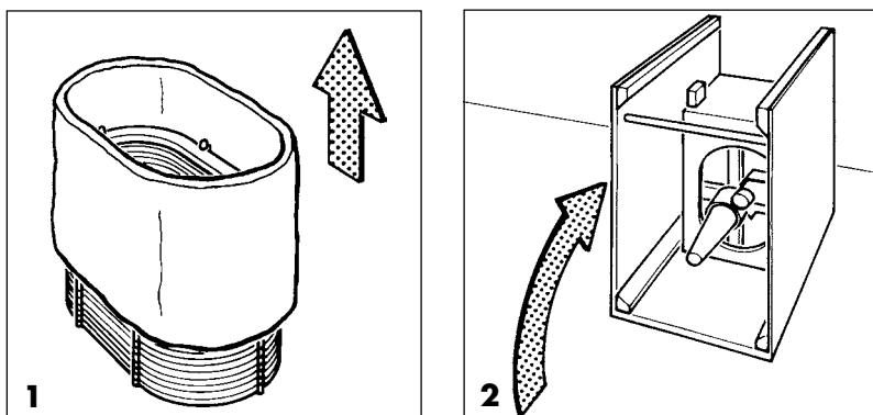
**Fig. 3** Withdraw the centrifuge from the coupling in a straight line.
